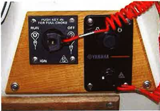
Hooked from the ignition to your life jacket, waist, wrist or thigh, this lanyard shuts off the engine and stops the boat if the operator is thrown overboard.
